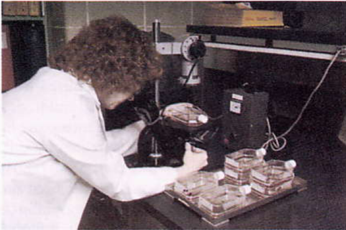
FIGURE 54-6 Inverted microscope used to examine cell monolayers growing attached to the inside surface beneath the liquid medium.
